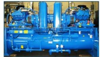
**Cogen:** Also known as "Co-Generation", this solution essentially works like a car engine. Natural gas is fed into the Cogen unit, and it not only generates electricity, but also utilizes the excess heat for domestic hot water needs.
